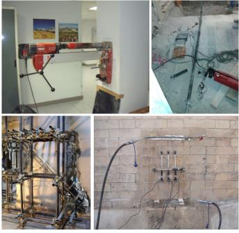
The *PRiSMa* Lab also acts in the area of the quality control of composite materials employed for structural strengthening, performing in situ pull-off and shear tearing tests.
