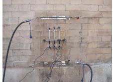
The *PRiSMa* Lab also acts in the area of the quality control of composite materials employed for structural strengthening, performing in situ pull-off and shear tearing tests.
